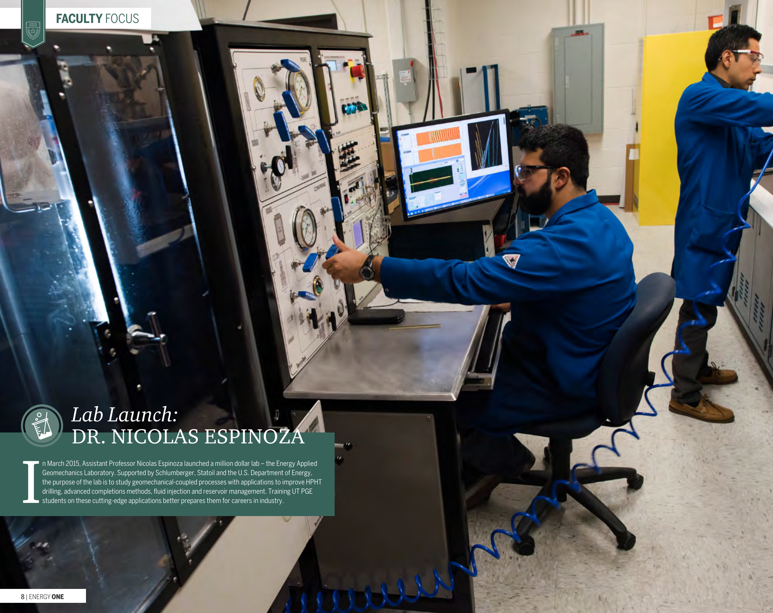
Stage of Triaxial Cell – State-of-the-art machine produced by Terratek/ Schlumberger measures the mechanical and transport properties of the rock in-situ pressure and stress for ultra-deepwater drilling and hydraulic fracturing
